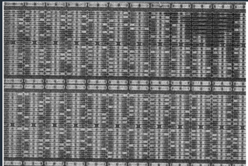
Fig. 5. 0.21 \mu\text{m} 2T memory cell content extraction
